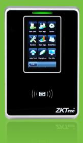
SC700 is a 125 KHz proximity access control terminal incorporated with 3" TFT LCD. The color display and touch screen operation offer a user-friendly and easy menu management.
